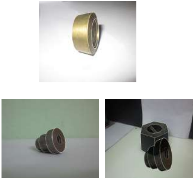
Fig. 6 Alignment of wireframed models with the objects in real images.
